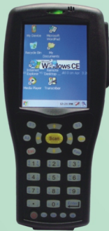
Model: ACM319A-HF HF Handheld Reader & Writer, Support ISO14443A/B/15693 Tags
